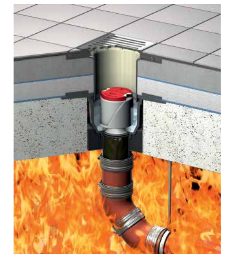
A fire on top of the ceiling expands. The intumescent mass in the odour seal to completely block the drain
